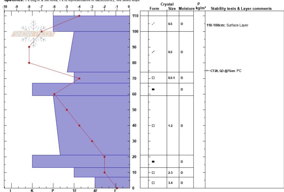
Notes: Pit was done where a isolated pocket of wind slab had developed from previous NW/SW storm.
