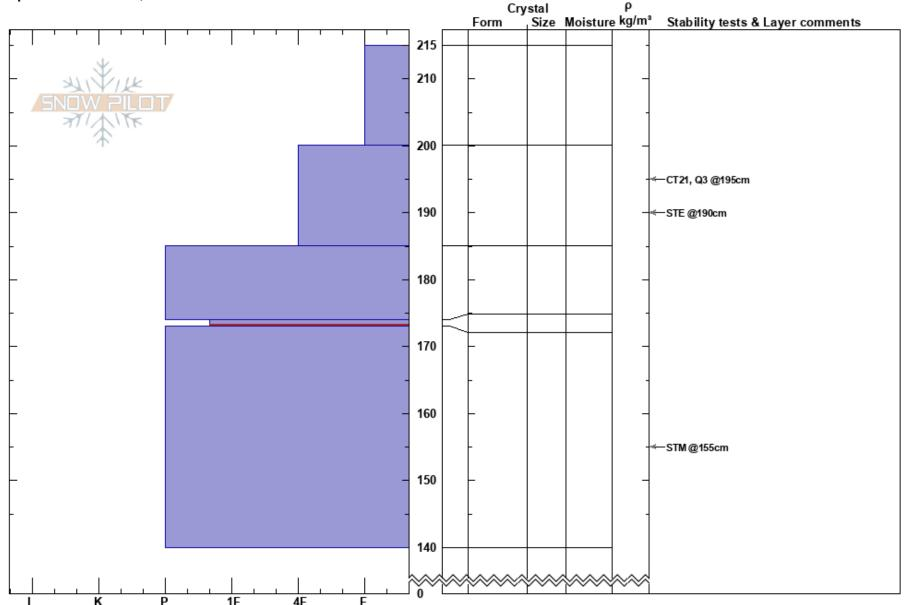
Notes: Hasty Pit dug with limited tests dug due to deteriorating weather. No apparent signs of instability in the pit. Only naturals observed were caused by solar input.
