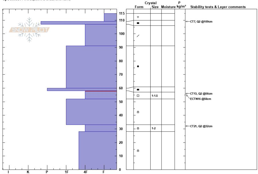
Notes: This pit was dug in the flank of a recent persistent slab avalanche. We got stable results in our stability tests on the layer the slide failed on. This is likely due to the layer having already collapsed.
