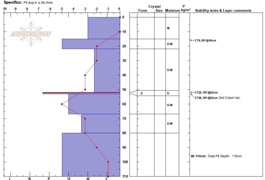
Notes: Pit was dug in lightly skied terrain in order to gain further understanding of what 1.5-2.5" of rain is going to do to the ski area snowpack at Stevens Pass Ski Resort. A Snowpack Percolation Test was also performed to investigate where water will pool versus run horizontally.
