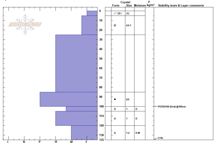
Notes: Propagation to end of column started along the facet interface and then progressed into the lower facets. It took a lot of effort to move the column downhill once the test was
