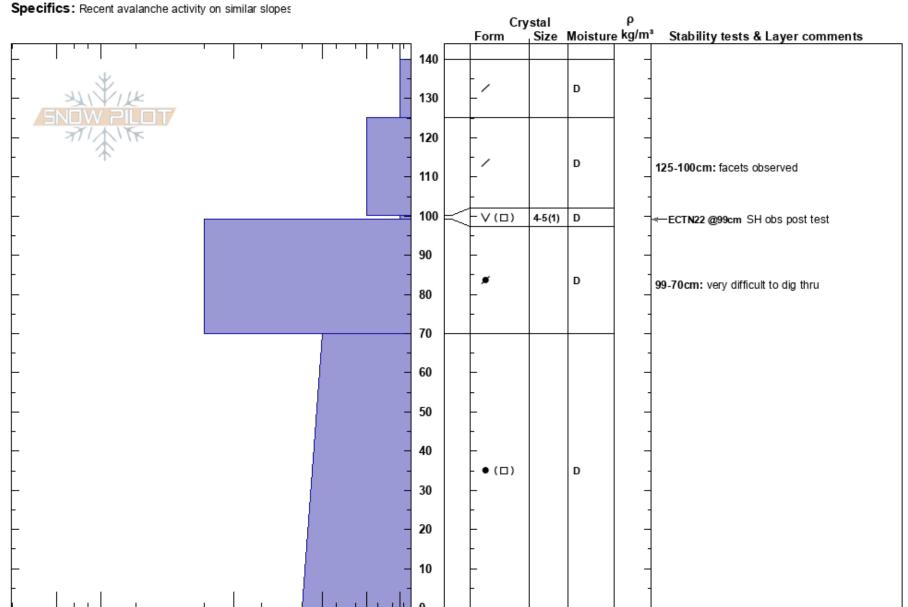
Notes: This saddle is in a windy location - probing for a pit site found variable snow depths ranging from 200cm to 50cm within a distance of only 30m.
