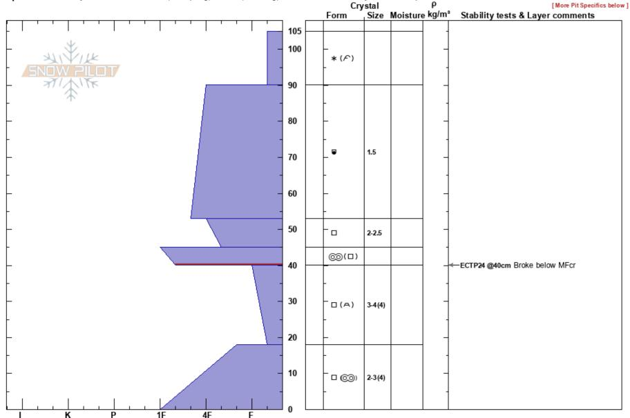
**Notes:** ESE Aspect. Avalanche remote triggered by Skier approx. 300' to the east. I was on lower downhill facing flank for the profile. Snow depth and structure consistent on entire slope. Failed on MFcr and stepped to ground. Additional Pit Specifics: Recent avalanche activity on different slopes
