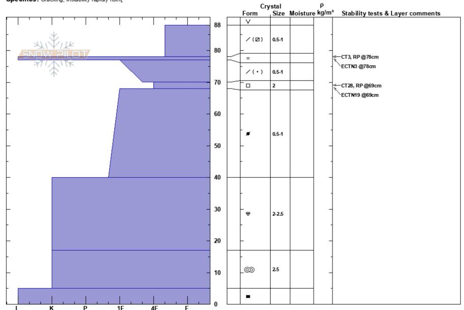
Notes: Over 1 hour while digging pits, the wind picked up to moderate and there was heavy wind transport. Swd reactivity quickly became touchy with 10-15cm slabs propagating on small test slopes.
