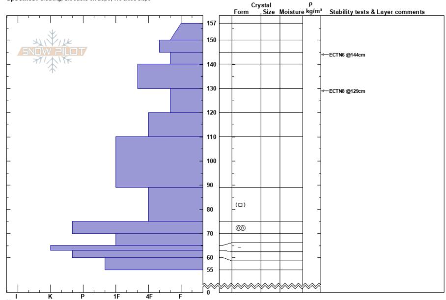
Notes: Very isolated and minor cracking. Could get the cracks to travel up to a meter in a couple of rollovers of small test slopes. These were windslabs (~28 cm below snow surface) from 24 to 36 hours ago as well as more recent storm slabs (10-15cm below snow surface). The ECTN results reflect these layers.
