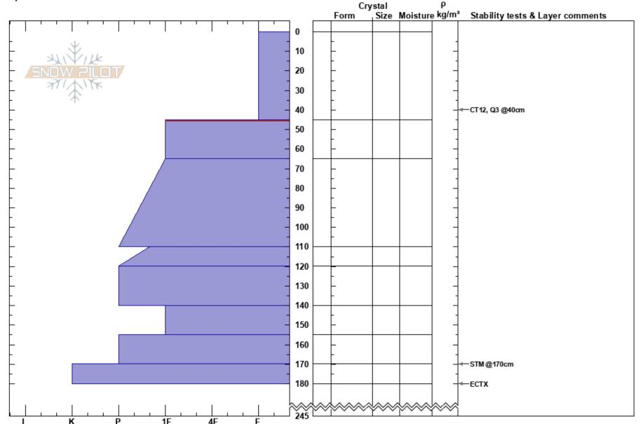
Notes: Did not have rutschblock cord for ECT. Cut with a saw on both sides so, the test may be inaccurate due to not being entirely cut.
