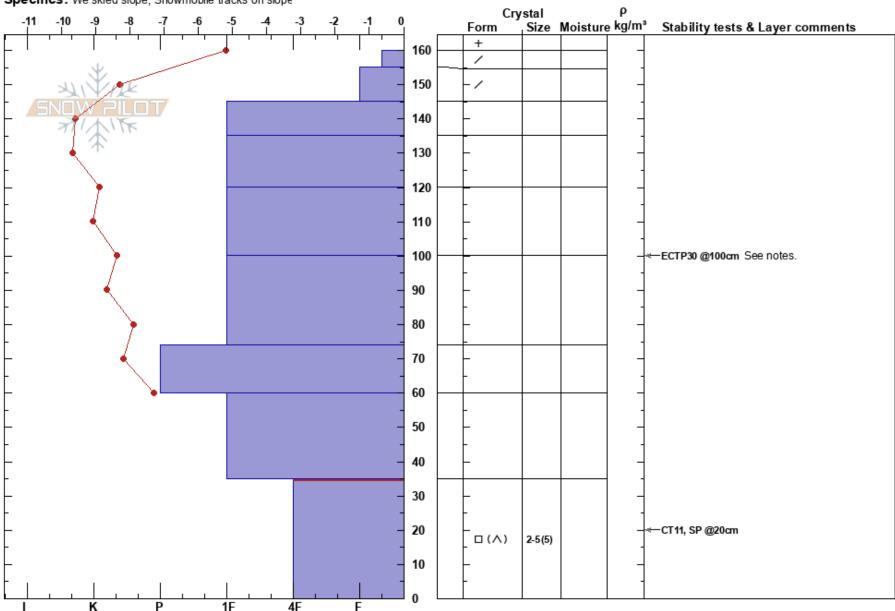
Notes: During the ECT, I cut down 120cm to isolate the back of the block. After the test (ECTP30@down60cm) I pulled the block off and another 65-35cm block from below came with. The intial propgation had stepped down in a non-planer shear to the stiff slab below.
