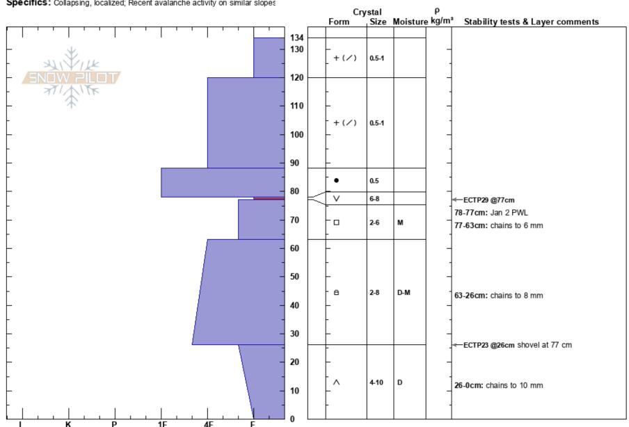
Notes: Pit dug in open, wind protected terrain just below treeline. ECTP-23@26cm was obtained after removing the top of the column following the ECTP result at 77cm and the loading steps were restarted from the beginning with the shovel placed at 77 cm in an effort to test step down potential following an avalanche initiation at the 77 cm height.
