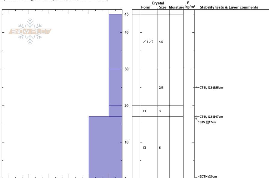
Notes: hard slabs currently developing. pit dug in the crown of a small slide set off by a 2# shot. AE HS R1 D.5 O. The slide broke at the 17 cm layer.
