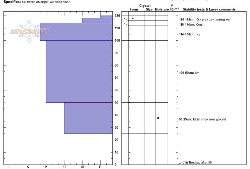
Notes: Stable conditions observed at this location, at the bottom part of a slope with a western aspect. Conditions may be different at the top of this slope, but the snow cover there seems less than at the pit location.
