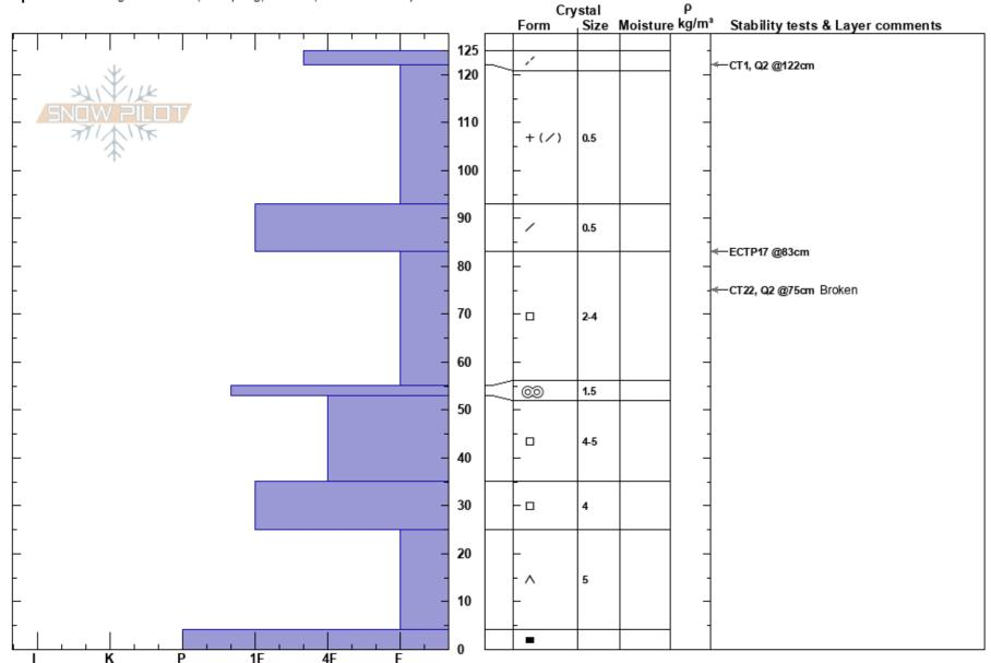
Notes: Pit dug in area where we have done a lot of work. Possible that some of the lower layers are old compaction work starting to rot out.
