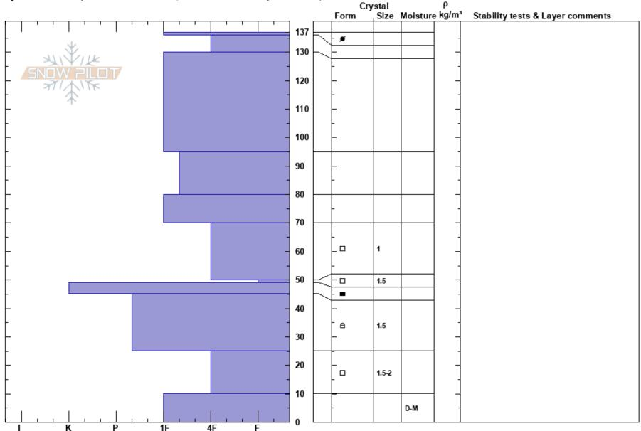
**Notes:** Crown face of snowmobile triggered avalanche. Triggered from low angle terrain in the run out zone. Alpha angle was 23 degrees. Heavily wind loaded. Crown averaged 2-3 feet deep was 6 feet deep in some places.
