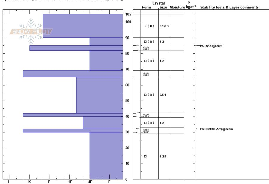
**Notes:** This profile has multiple layers of concern. All the crust/facet combinations are troublesome. The crusts are 3 to 4 cm thick and very supportable. Each could be a bed surface on its own. However, future loading will determine which one and how deep failure occurs. It seems this matrix could support quite a bit of weight before it goes.
