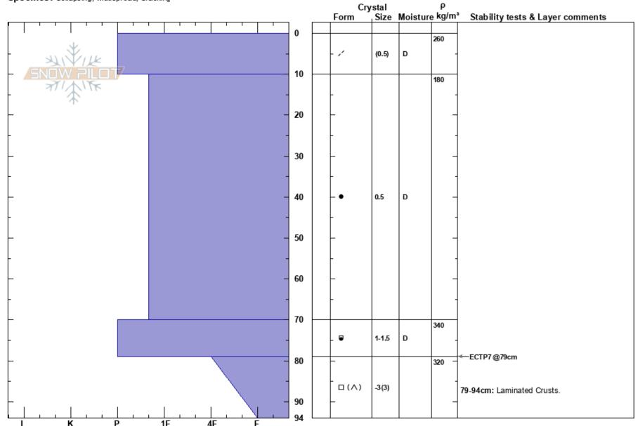
Notes: HS typically 50-75, highly variable and wind scoured. Observed numerous shooting cracks and settlements approaching test location.
