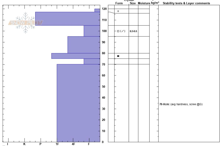
Notes: Profile 10m to gunner's right flank of avalanche. ASu-HS-R2.5-D2-O. Crown was estimated 1-3 feet thick based on size of chunks in debris, reloaded by wind and snow since avalanche.
