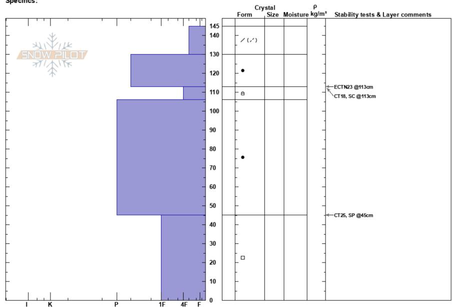
Notes: The weakest interface is >1m deep in the snowpack, but several weak interfaces persist in the upper snowpack as well. A slide triggered in the upper layers would likely step down to the deepest weak layer, resulting in a very large and dangerous avalanche.
