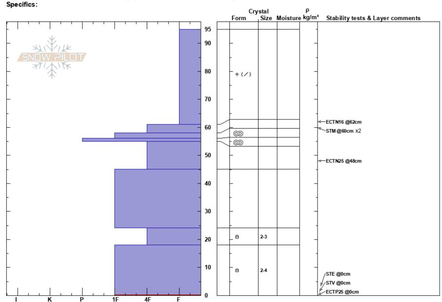
Notes: ECTP on the ground was not repeated. When pulling on the column during the second test it easily tipped over failing at the ground. The back wall of the ECT's showed a clean cut to the ground. Facets at the bottom of the snowpack were beginning to chain together but still showed poor structure. J. Reddy was the scribe.
