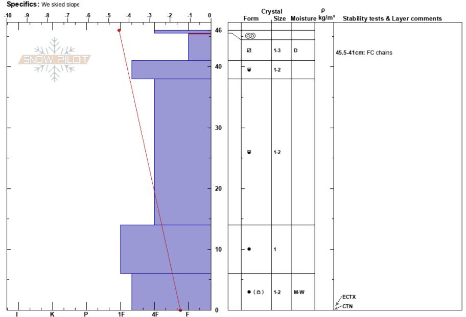
Notes: Pit dug in below treeline avalanche path. We also did 2 Loaded PST tests. 10cm of an artificial slab that was 4f-4f+ hard after 1 hr of sitting. Both tests resulted in a slab fracture failure 30cm into the cut.
