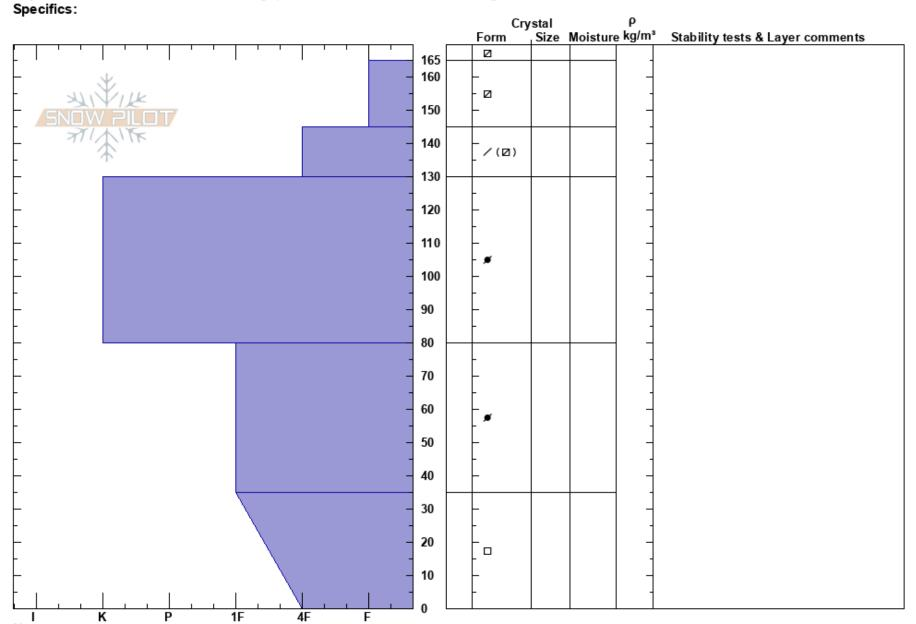
Notes: The Knife layer was so hard my saw struggled to cut a good column. No snowpack tests preformed. This area is heavily wind-loaded.
