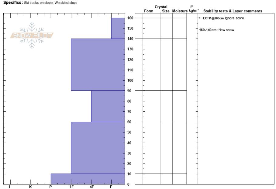
Notes: Tapped ECT and Compression up to 30 without fail. Using a shovel to wedge the back of the column, we did get failure on the Compression and ECT columns at 90 cm above ground at the top of the 4F layer. For the compression test, the block sheared ad popped out with a bit of energy. The ECT failed at exactly the same depth and propagated across the entire 1 meter wide column with little/no energy.
