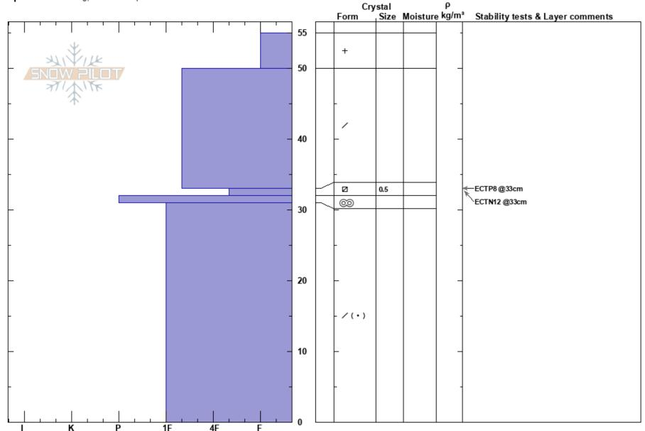
Notes: ECTs results were inconclusive - some tests propagated across the entire column while some arrested halfway through the block and slab fracture observed.
