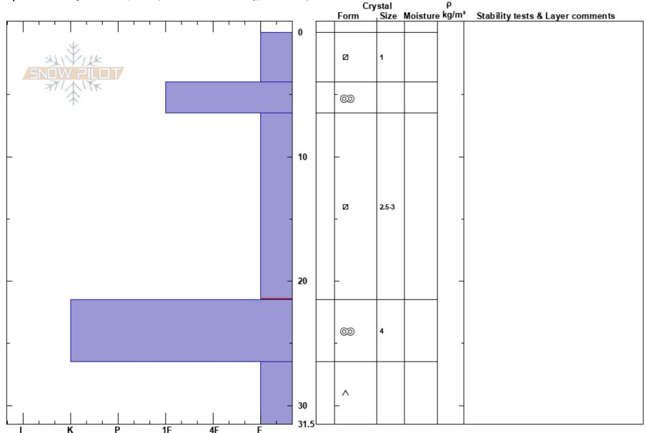
**Notes:** showing difference of a pit fully shaded and one exposed to a few hours of sunlight but still north. As aspect becomes more easterly and exposed to sunlight, the crust near the surface thickens.
