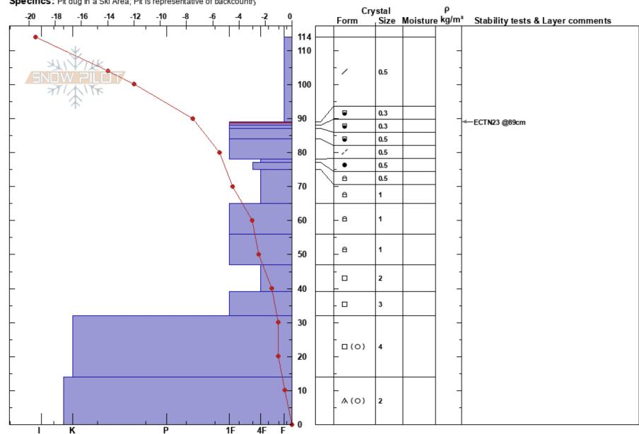
Notes: 32 cm layer could not be cut by the saw for testing. All Tests were cut down to this layer, but no further.
