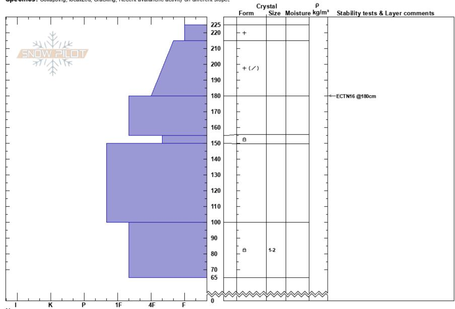
**Notes:** Recent 1-2' soft slab avalanches triggered on wind loaded slopes. A large natural occurred on ridgleine above this pit 1/4 mile to the north between the time we left this pit (1415) and 1530. It was on a heavily wind loaded slope, broke from a cornice fall 4-8' deep on facets near the ground. R3D3-N-O
