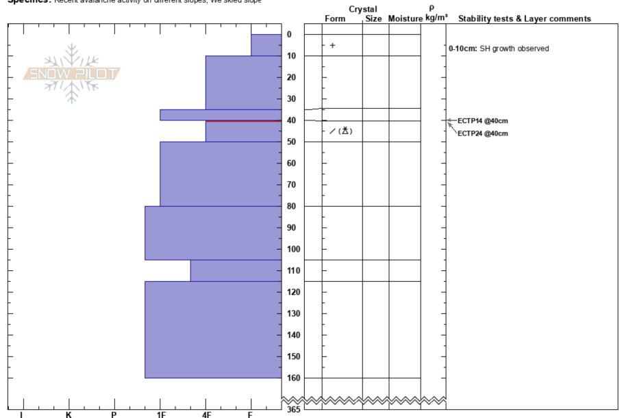
**Notes:** Pit dug on slope below the start to the cody bootpack. Problem layer showed repeated propagation failure. Interface was a density break that included graupel and possible faceted grains.
