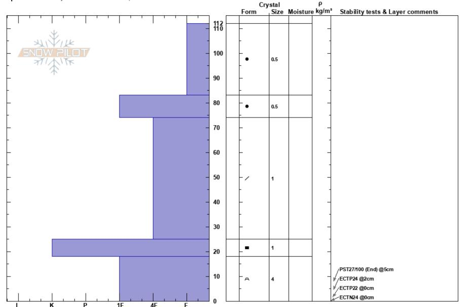
Notes: This is a fracture line profile performed on an slide that occurred right off State Highway 110A, on the east side of the road, across from Niagara Gulch. The approximate width was 50', track ran 80', and the length was 100'. The bed surface was a grassy slope, above a creek, with an unsupportive base.
