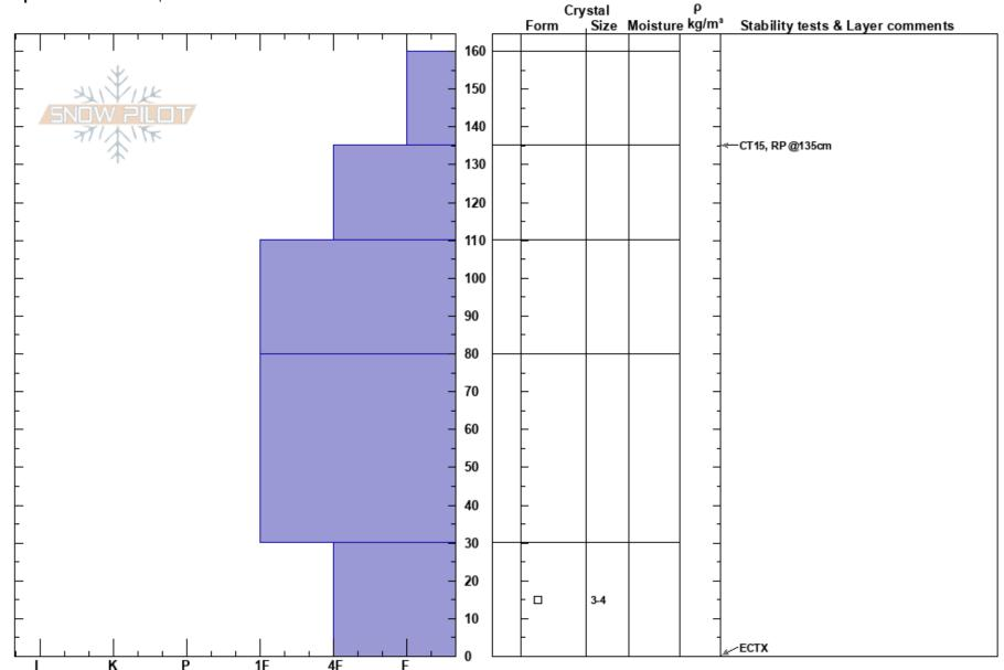
Notes: HMH SRSC Recon. No Cracking, Collapsing, Whoomphing. Similar slope was controlled with explosive with no results.
