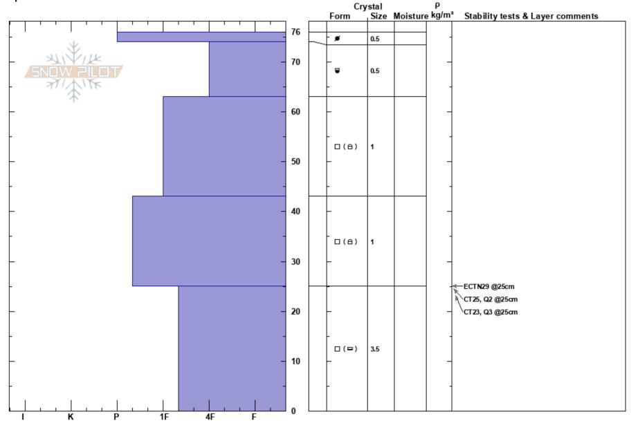
**Notes:** Depth hoar crystals found at the bottom of the snowpack. Some rounds and rounding edges within the crystals were observed. The resistance is 1F-. These crystals are slowly gaining strength.
