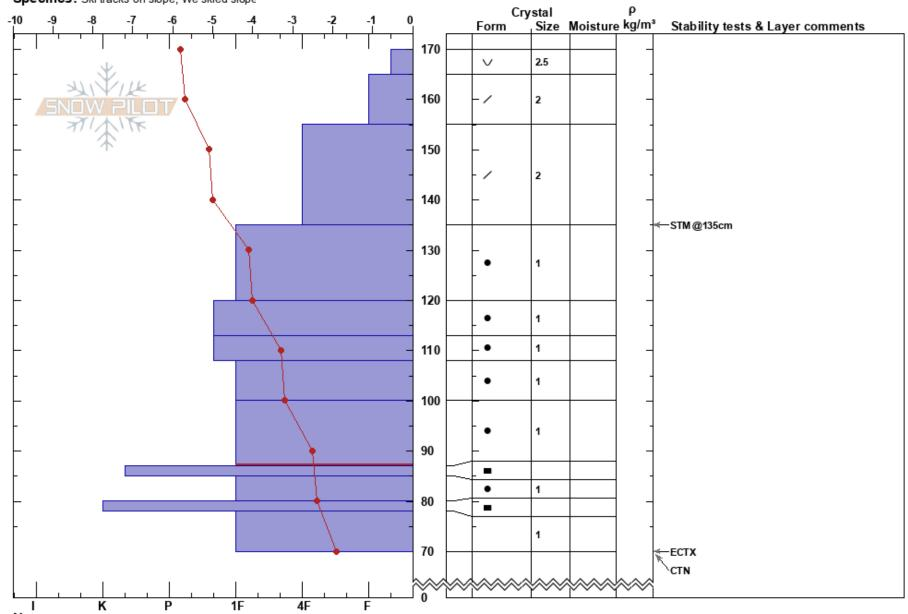
Notes: Pit location was sheltered by rock band above on ridge. Slopes to the right and left without the rock band shelter had cornices and were being wind loaded at time of observations. Test results ECTX and CTN
