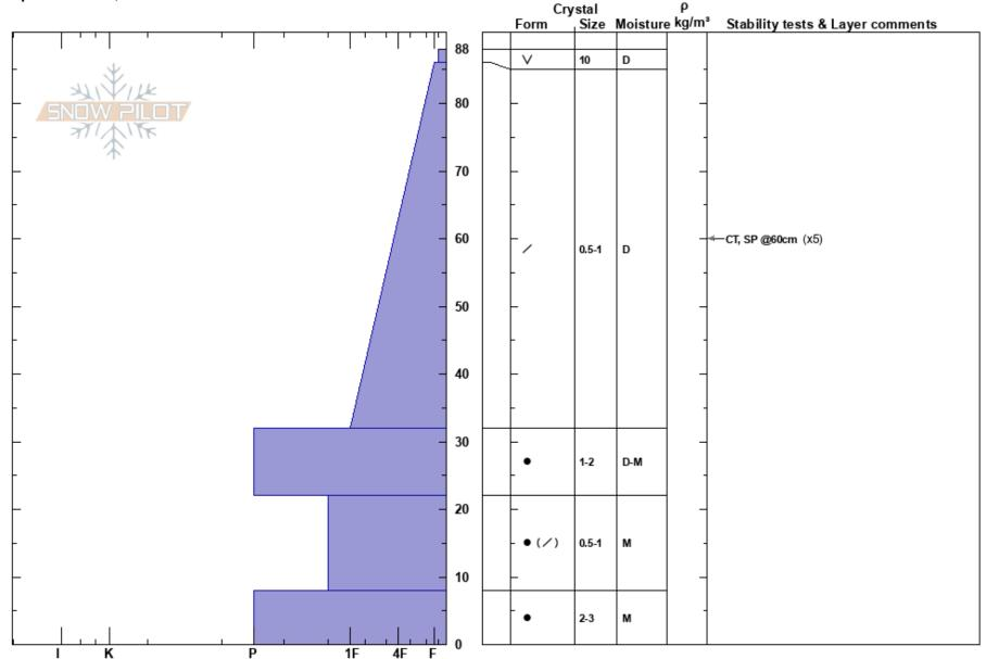
Notes: SH is now at least 2 cm thick with many crystals exceeding 12 mm. Difficult to ID failure layer in CTs: very soft, very thin (previously buried SH? Unsure.).
